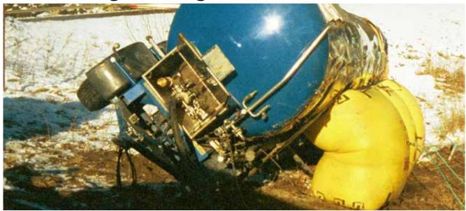
MFC Survival offer a comprehensive range of 0.5 bar pressure high lifting cushions designed primarily for the recovery of larger vehicles.
